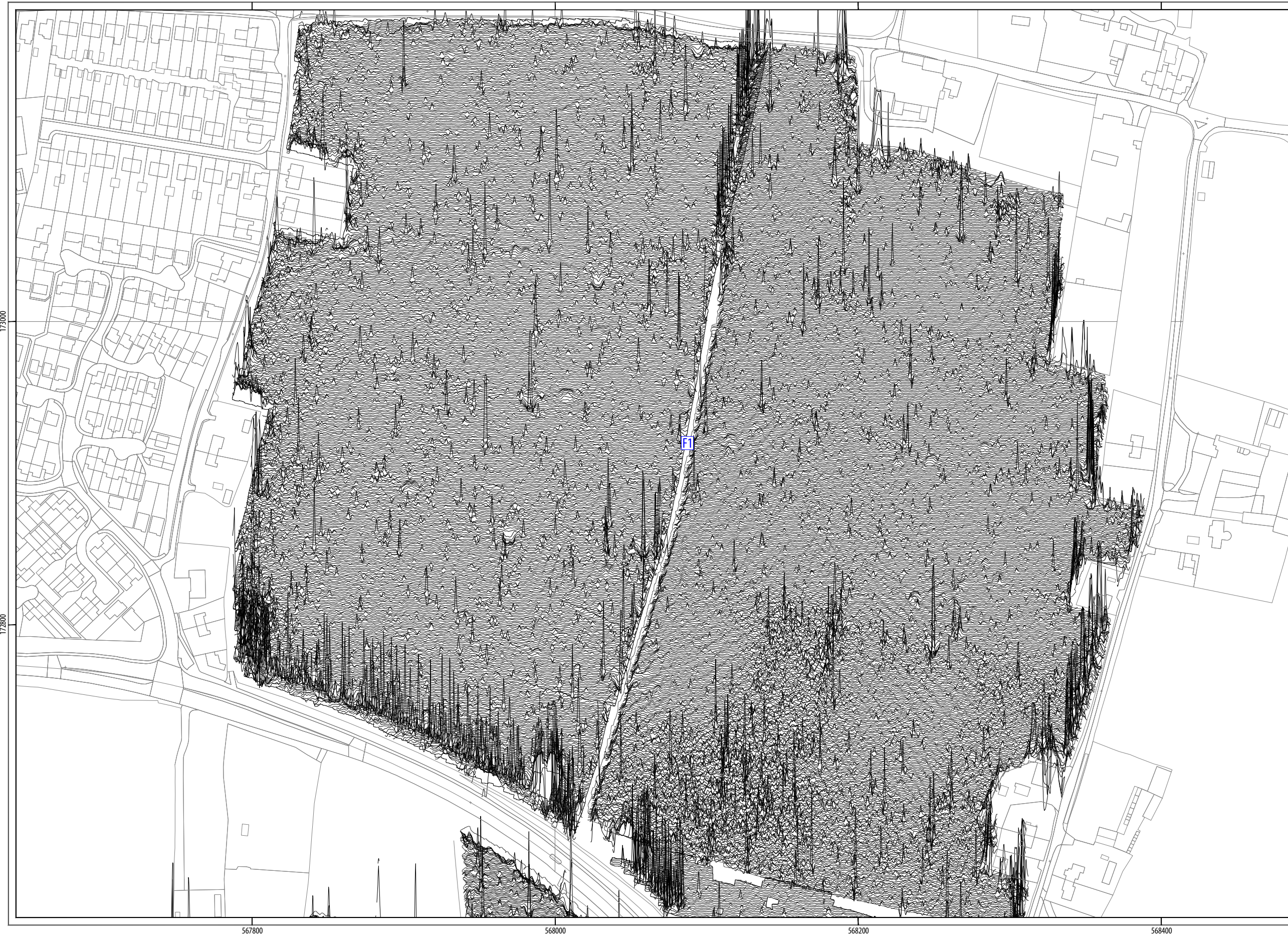
ILLUS 13 XY trace plot of minimally processed magnetometer data; Sector 1
