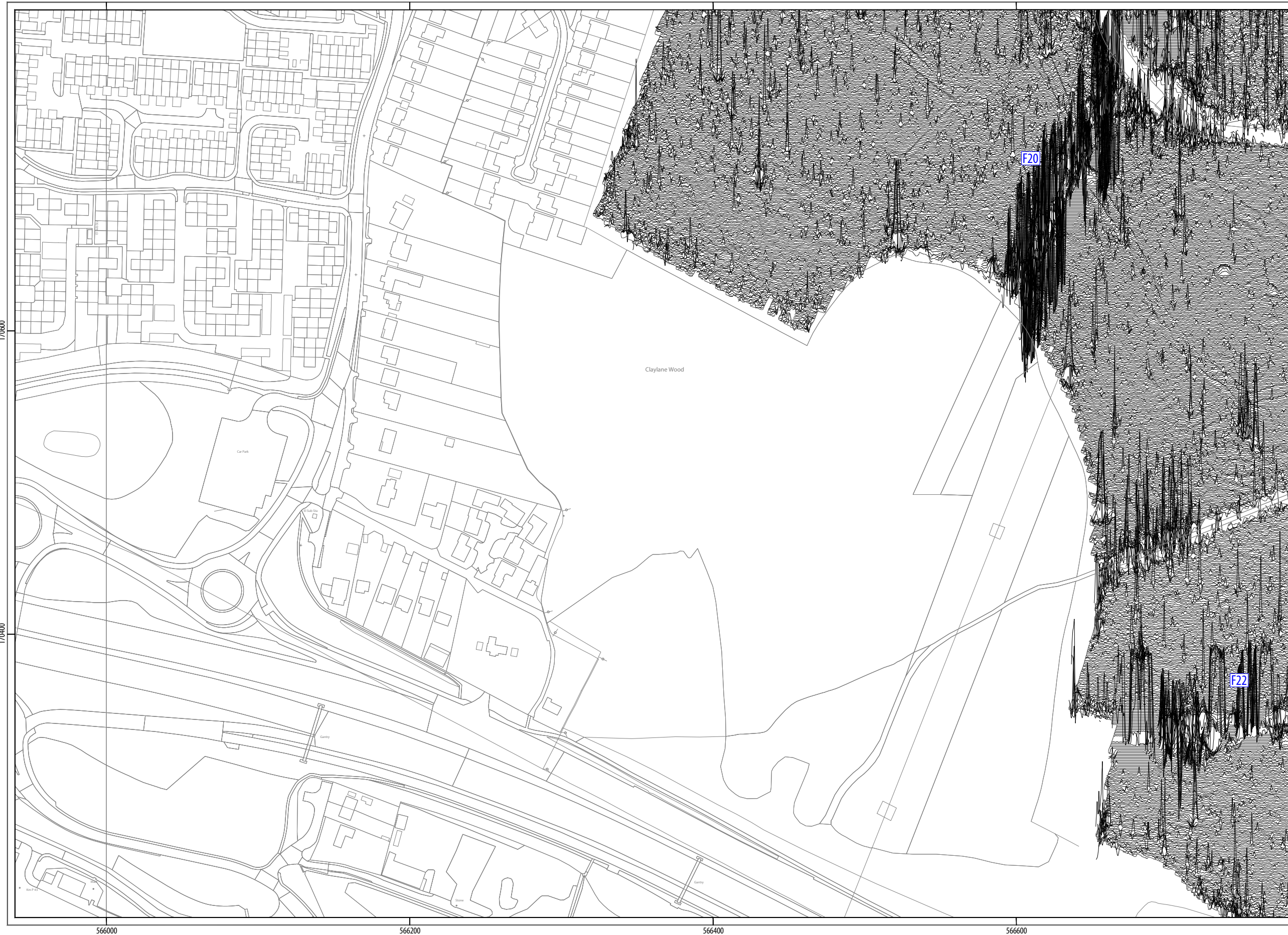
ILLUS 37 XY traceplot of minimally processed magnetometer data; Sector 9
